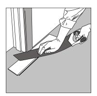
**Door mouldings and skirtings:** Put a panel (with the decorative side down) next to the door moulding and saw as shown in the figure. Then slide the panel under the moulding.
