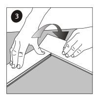
**3. Connect additional panels** Next panel is an A-panel. Again, press the long side of the new A-panel at an angle against the short side of the previous B-panel and fold down. Continue like this with as many panels as may fit along the starting wall.
