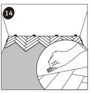
14. Put in spacers Put in spacers between the flooring and the wall to ensure a expansion gap of 8 -10 mm
