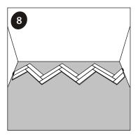
8. Continue with the B-panels Now work in the opposite direction, from the right to the left and install all the Bpanels in the second row. Finish with a piece of panel cut to size (step 5).
