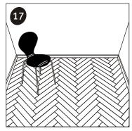
17. Spacers and skirting Remove the spacers and cover the expansion gap with skirting boards or beadings.
